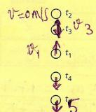
11. Assume that the downward direction is positive. For each time shown on the diagram, determine whether the direction of the velocity is positive, negative, or zero, and whether the direction of the acceleration is positive, negative, or zero. Record your answers in the table using the symbols +, -, and 0.
