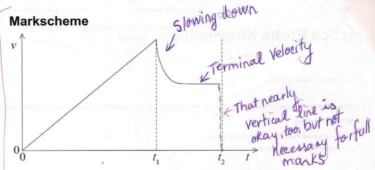
straight line to water surface; (allow a slight curve within 10 % of  $t_1$ ) clear decrease after hitting surface; (allow straight line or concave curve as shown, do not allow convex curve)
